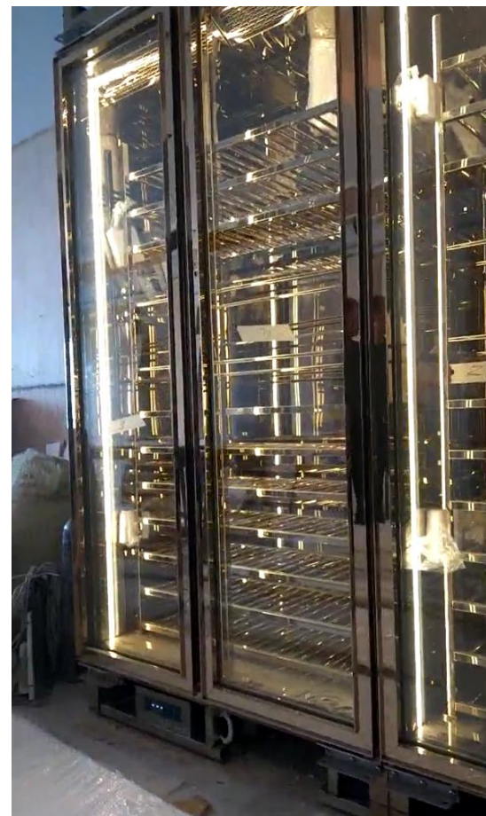
Stage 1 The bodies and the bases of the cabinets are reassembled, waiting for the doors to be installed.
